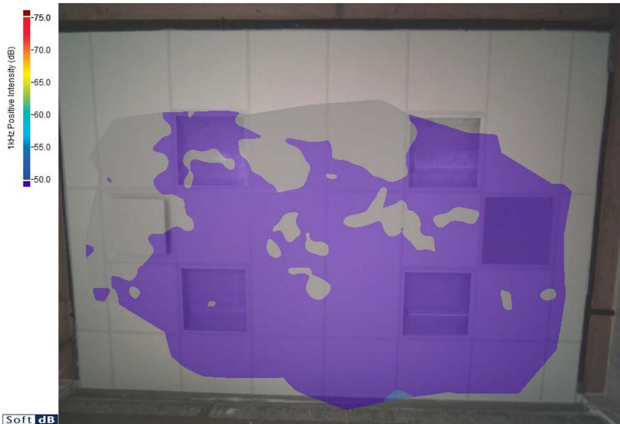
**(4c) With Plenum Barrier** - This ceiling system is comprised of 1-inch-thick, stone wool, ceiling panels with a CAC 22 and NRC 0.95. It is suspended using the same grid. A double-layer, stone wool, plenum barrier is installed above the partition along the bottom of the image. Overall, noise levels have been decreased an additional 20-25 decibels (dB) compared to using the mineral fiber ceiling panels alone.
