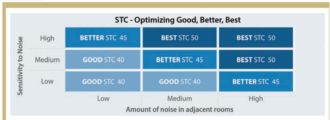
*To select the optimal sound transmission class (STC) rating for the walls between rooms, both the potential for noise in the adjacent room and the sensitivity of the room's occupants to noise should be taken into account.*
