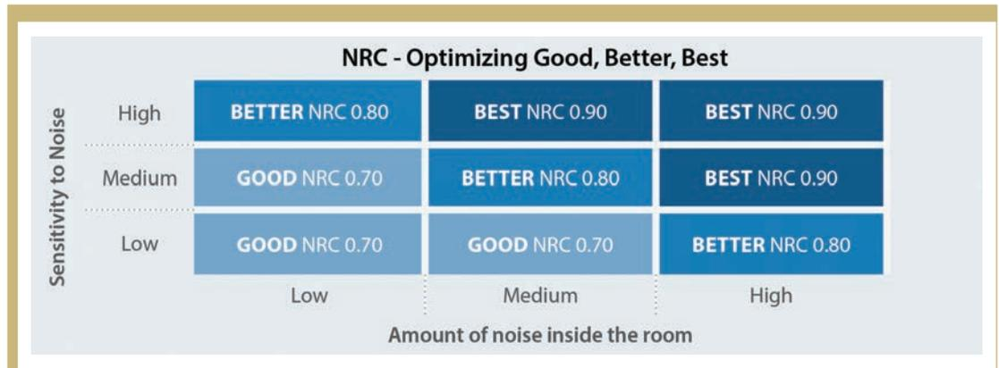
*In selecting the optimal noise reduction co-efficient (NRC) for the ceiling in a room, one must consider both the potential for noise inside the room and the sensitivity of its occupants to noise.*
