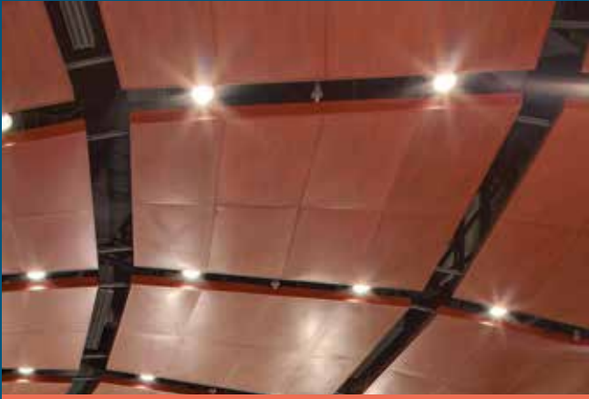
SpanAir Torsion Spring metal ceiling panels are each a trapezoidal shape and connect into 30-inch by 5-foot tapered pods, suspended at the proper angle and aligned with equal spacing for a uniform appearance.
