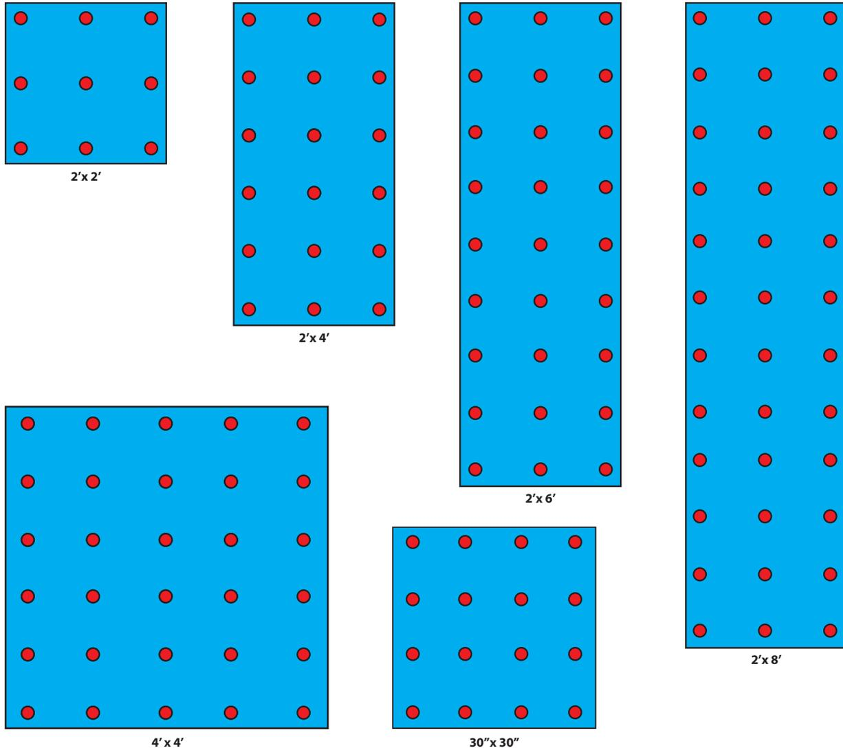
Larger panels should be bonded with a golf ball size mound of adhesive located at the corners of each square foot of panel space. A trowel can be used to apply the adhesive instead of golf ball size mounds, but must select a trowel that will form ridges or beads of adhesive that will allow the adhesive to bridge the gap of the panel to the flatness of the intended bonding surface. Failure to bridge the adhesive from the panel to the intended wall/ceiling surface may cause panels to fall.
