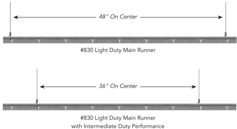
*Note: When such installation modifications are performed, only the performance capability of the main runner, and not the actual ASTM C635 rating, is increased. Also, these recommendations for increasing the performance capabilities of main runner components apply to Rockfon® products only.*
